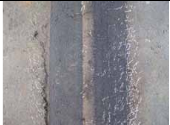
Plan view of test sections, note vertical asphalt and diagonal in plane shear cracking
