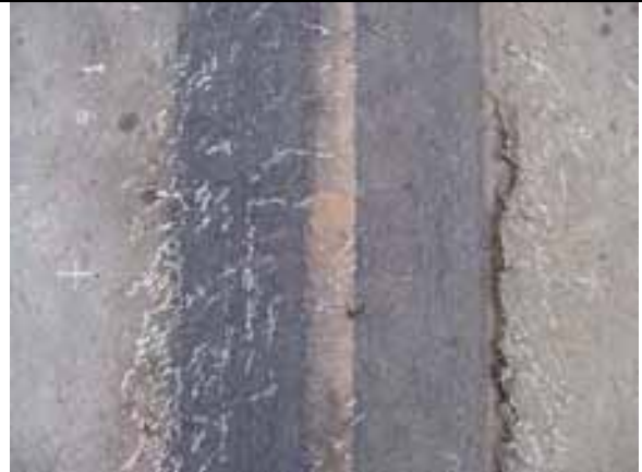
Plan view of test sections, note vertical asphalt and diagonal in plane shear cracking
