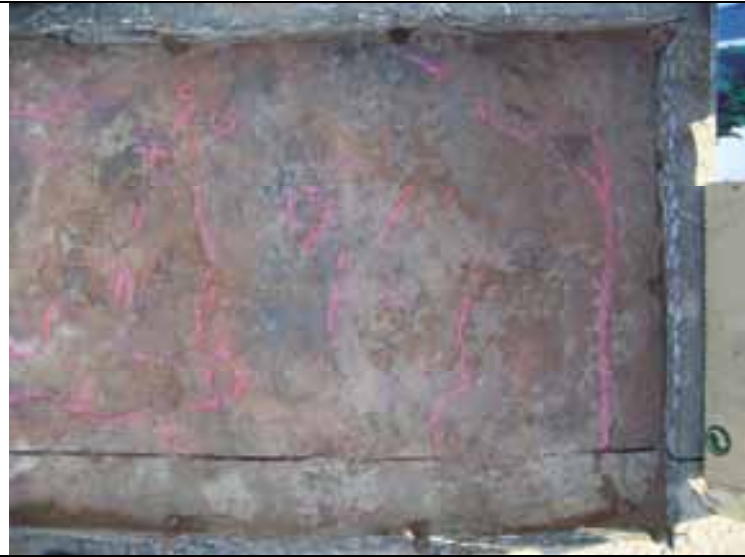
Top of CTB after extraction of HMA and side view of vertical HMA shear
