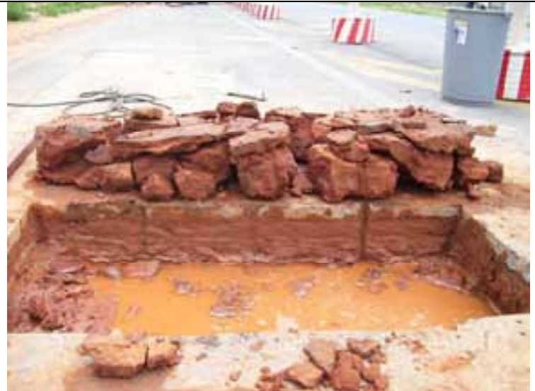
Side view of vertical HMA shear and plan view of CTB block before extraction
