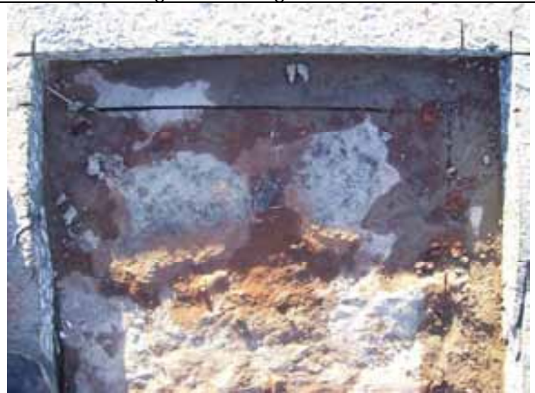
Plan view of HMA slab note smoothed surfaces. Top view of CTB block before extraction – Test pit 2
