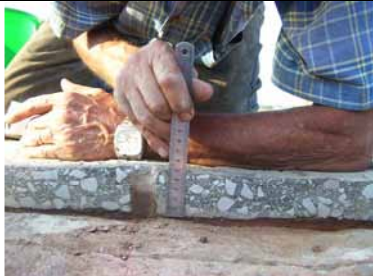
Side view of vertical HMA shear and plan view of CTB block before extraction
