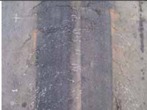
Plan view of test sections, note vertical asphalt and diagonal in plane shear cracking
