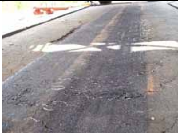
Plan view of test sections, note vertical asphalt and diagonal in plane shear cracking
