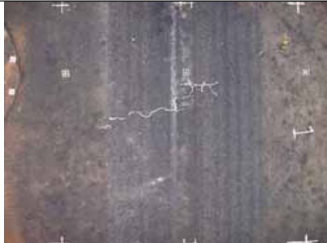
Plan views of test section with crack marked in white
