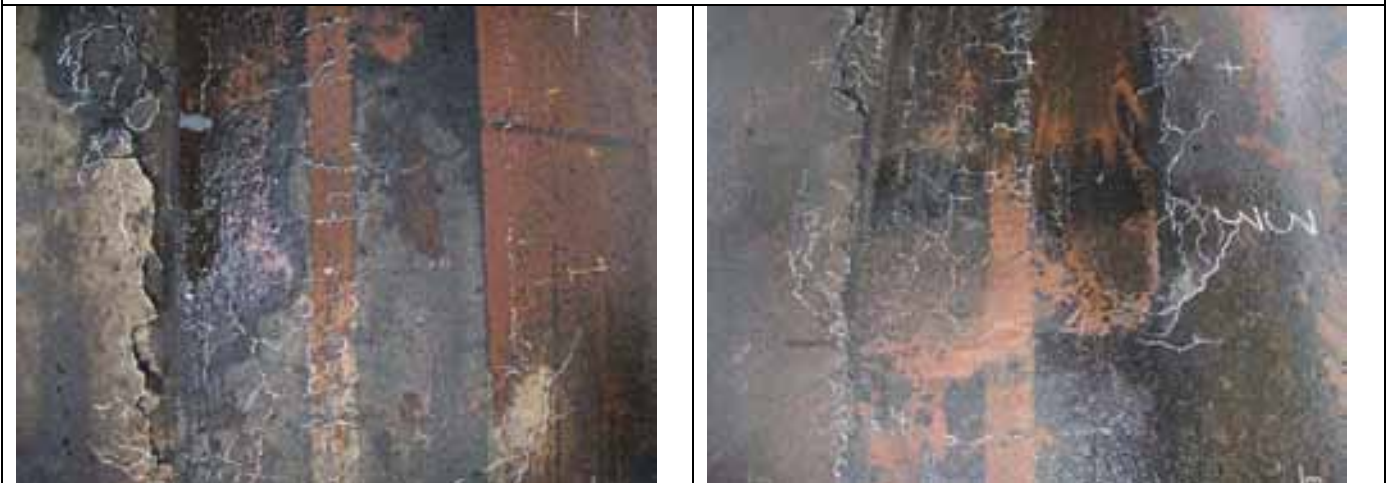
Plan views of base material pumped out of test section. Note extensive crack patterns
